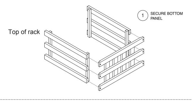
3. Attach the top panel to the top of each side ladder using the provided wood screws. (figure 2)
